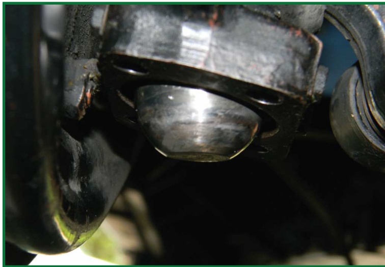
All traces of grease cleaned off the ball
