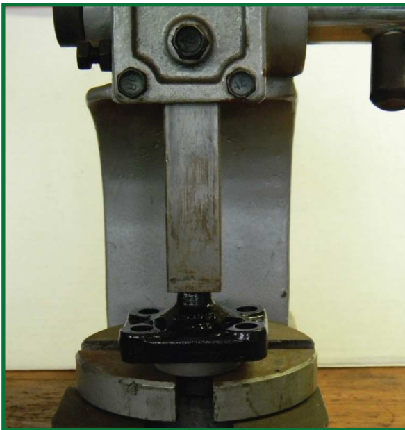
Pressing the phenolic cup into the cap
