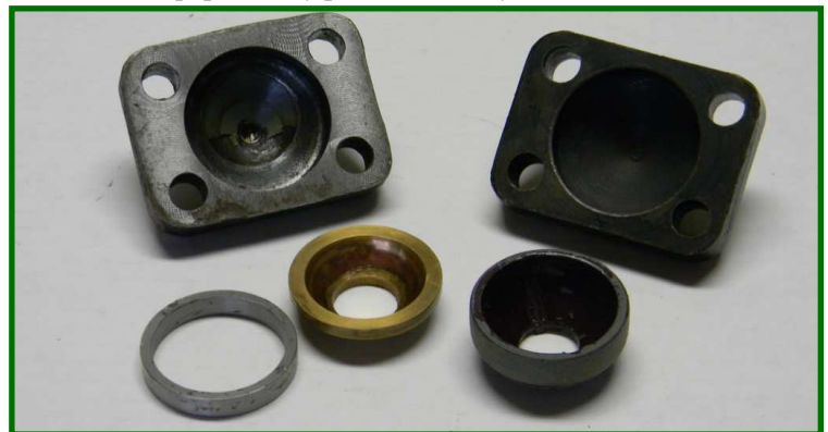
Spigot and brass cup on the left, with the new phenolic cup on the right
