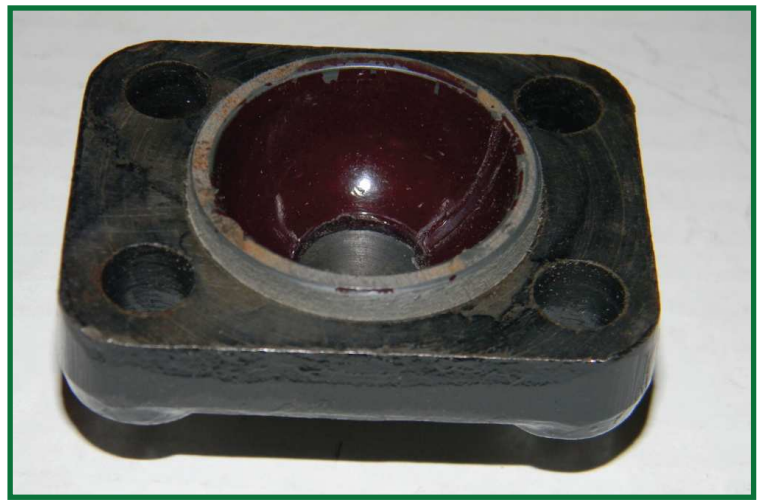
The new phenolic cup installed in the cap
